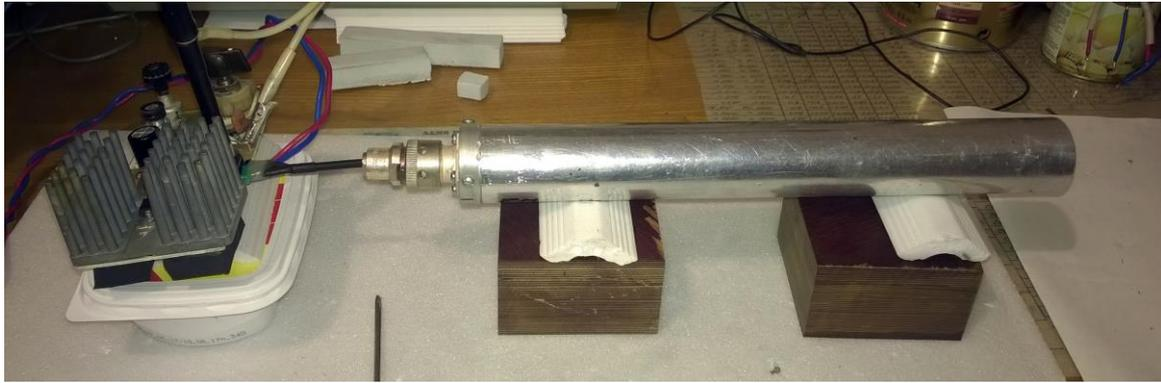
It is assembled from two long aluminum cylinders (outer and inner) and two aluminum washers. Internal space between two cylinders filled with toroidal ferrite cores. Permeability of toroids is 2000 $\mu$ . Sketch of the scalar gun (head) on picture below:
