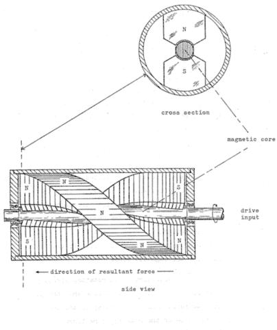
Figure 4. Linear Force Machine (magnetic)
