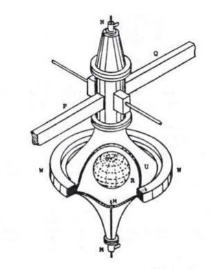
Figure 3. Cut-away view of reaction chamber "U" showing central plasma sphere R in equilibrium position.
