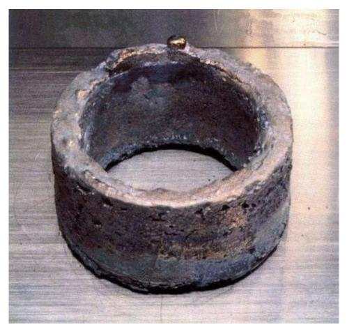
A ring of plutonium used in an atomic bomb core
