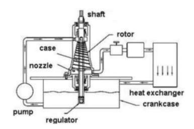
Figure 7. Principal scheme of Clem's device
