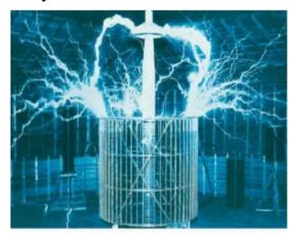
The flame-like discharge of an electrical oscillator giving twelve million volts which measure sixty-five feet across, Colorado Springs Laboratory.
