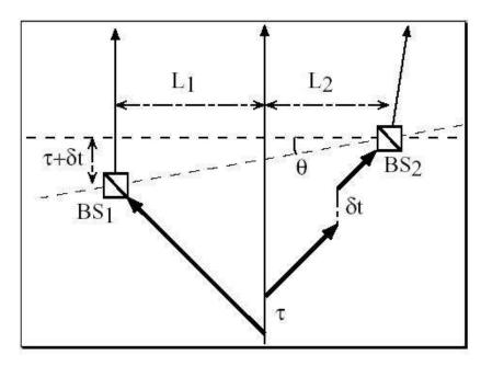
Time diagram of an experiment involving moving apparatuses and demonstrating that quantum correlations are independent of distance as well as of time ordering between the two measurements.
