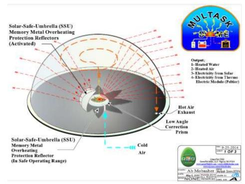
Its proprietary, non-electrical Solar Safe Umbrella reflects the sun's rays if its temperature reaches an unsafe level.
