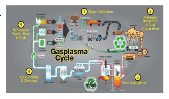
Advanced Plasma Power's advanced Gasplasma® technology today delivers 50% electrical conversion efficiency – twice that of conventional steam cycle technologies.
