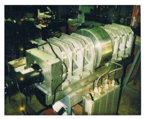
homopolar motor-generator. It was estimated that the cost of such an advanced electrical generator to be approximately the cost of installing smoke scrubbers on one coal-fired generating unit.
