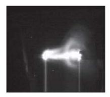
Plasma Spiral Toroid Around Electric Arc
