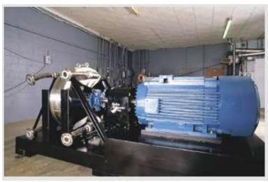
The rotor inside the Hydrosonic Pump<sup>TM</sup> generates shock waves to provide the energy needed to heat various liquids, such as organic salt used by the petroleum industry.
