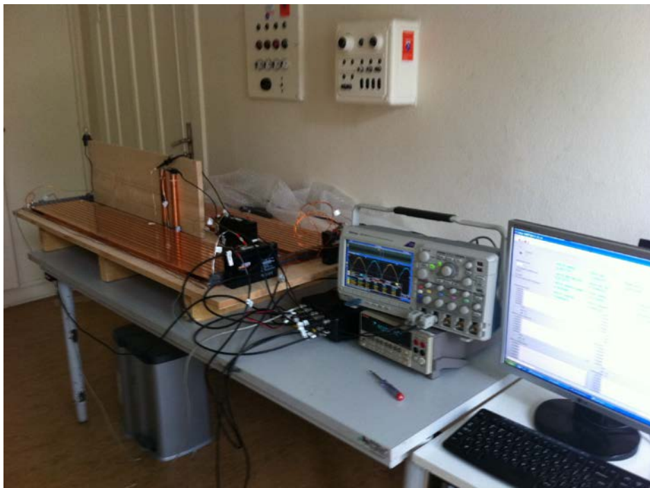
Figure 5. Measurements on the Coler replica with a Keithley 2000 DMM and recording and display with a Lab View program
